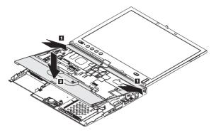
Note: After installing the upper case, route the wireless LAN antenna cable as shown in 3a.
