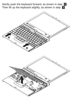
Detach the keyboard connector to remove the keyboard.
