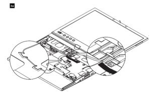
Note: For the models have BMDC-3, route the wireless LAN antenna cable and the Bluetoogh antenna cable as shown in <u>3b</u>.
