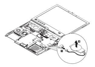
When installing: Make sure that the battery connector is attached firmly.
