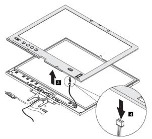
When installing: The replacement bezel should have adhesive pre-applied; therefore, remove the covering from the bezel to expose the adhesive, and then place the top edge under the frame, shown as 1, then push the bezel down and secure with the latches firmly. Be careful not to make the bezel touch the *Bluetooth* antenna from being deformed downward or inward as B. Make sure *Bluetooth* antenna is not deformed as A.
