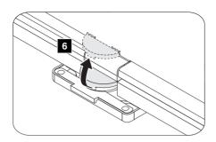
When installing: Make hinge cap parallel to LCD, and then pullup hinge to install well.
